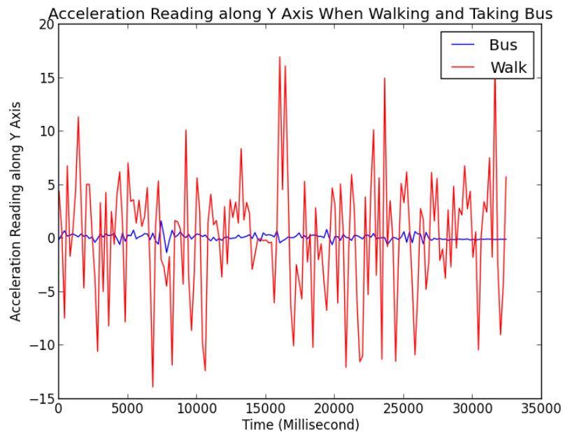
9 10 Fig 2. Acceleration Reading along Y Axis (vertical to earth) When Walking and on Bus 11
